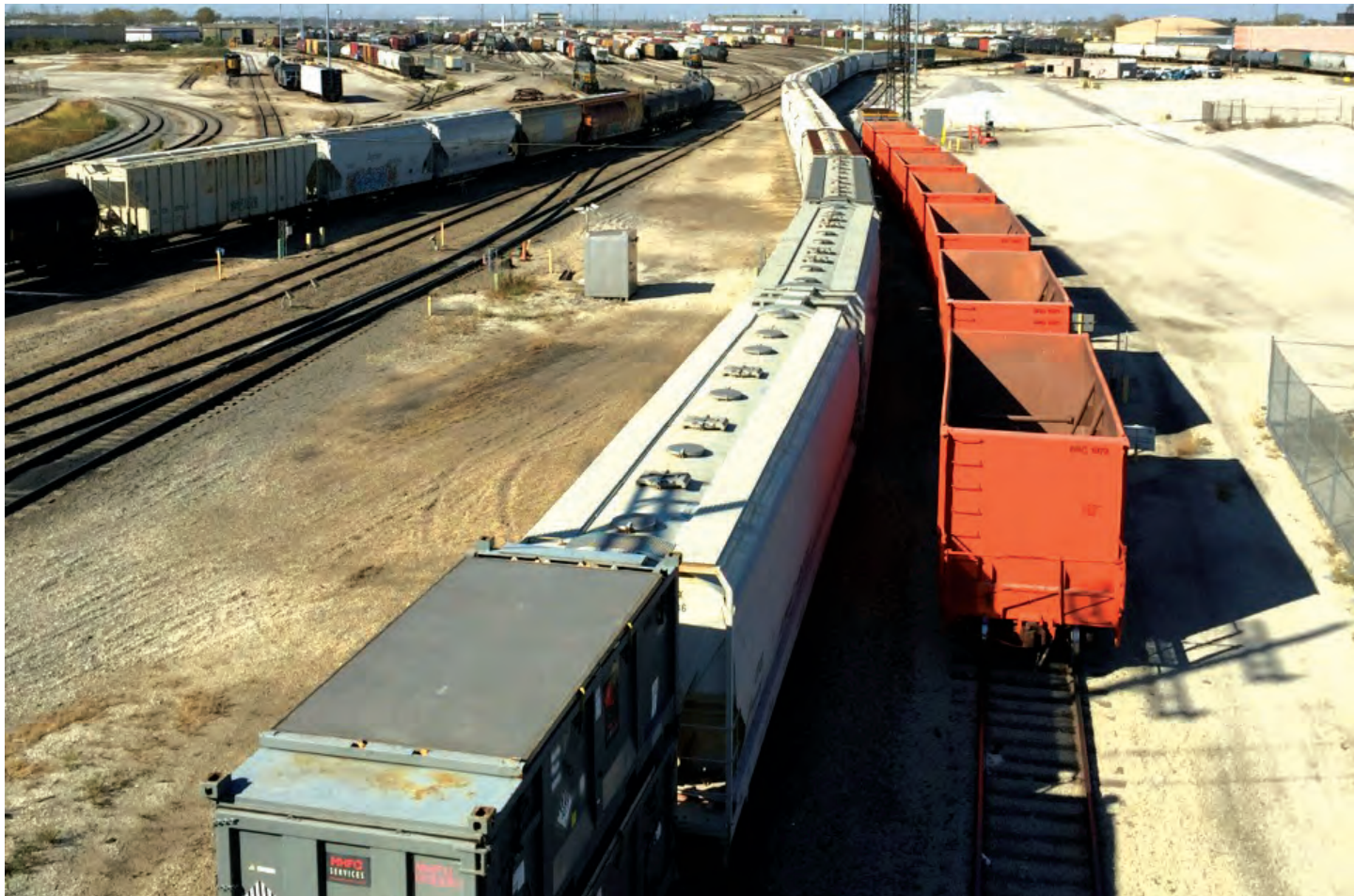
A The Belt Railway of Chicago—the largest switching terminal railroad in the United States—separates and classifies rail cars into rebuilt trains for 14 freight rail providers and dozens of private companies in the Chicago region at its Clearing Yard in Bedford Park.
