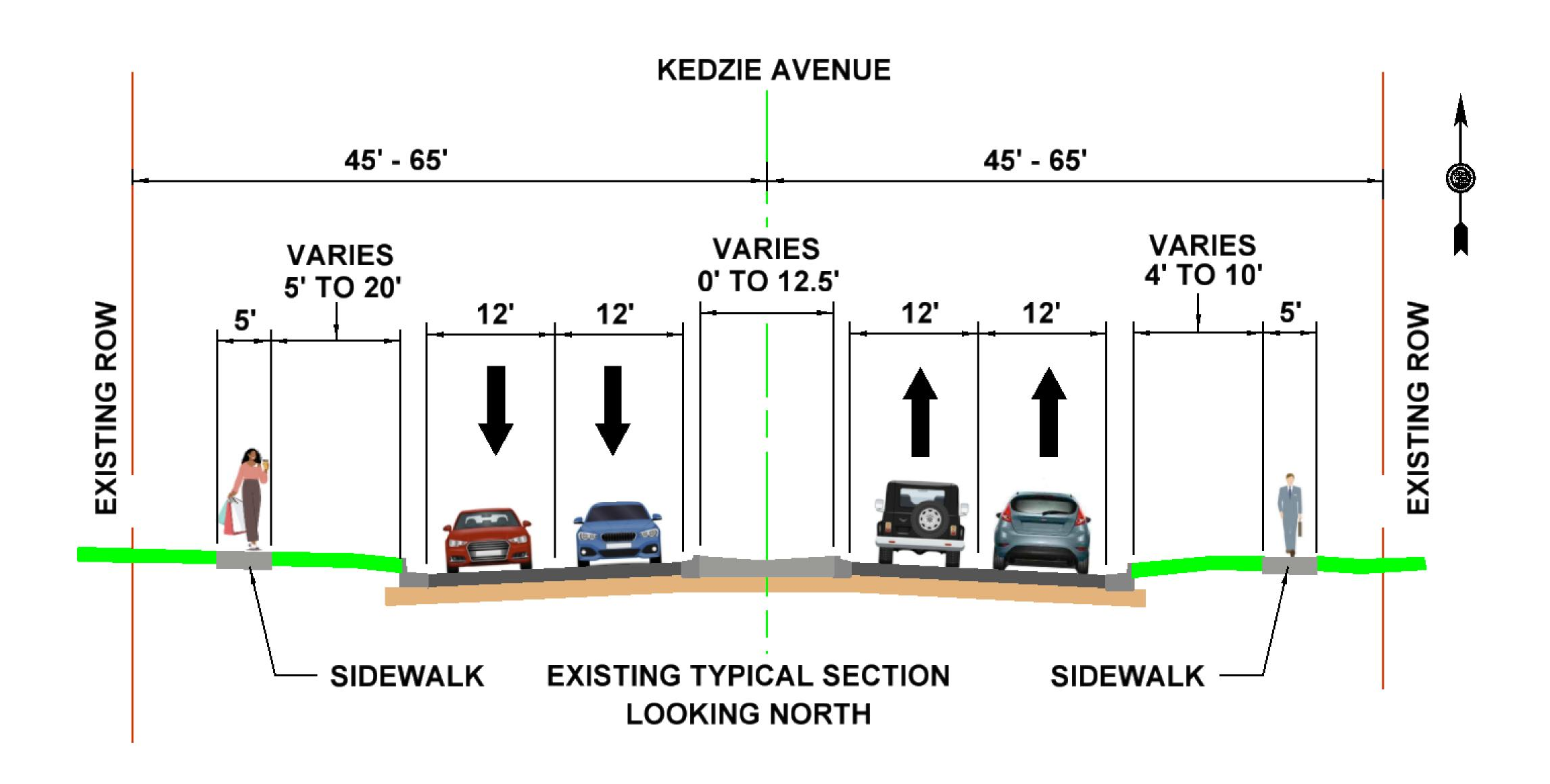
Most of the corridor consists of two travel lanes in each direction with left-turn lanes at intersections
